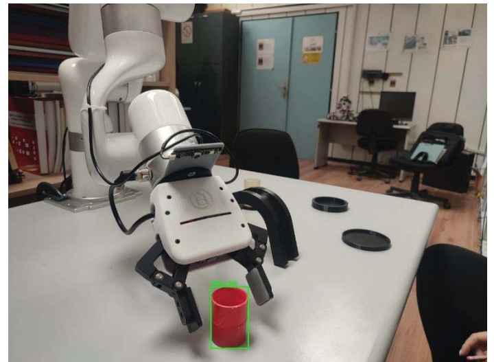
Fig. 2. xArm 5 with mounted camera doing manipulation task
